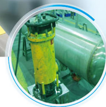
X光探伤仪 x-ray detector
